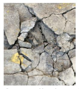
Concrete can withstand compressive forces very well but not tensile forces. When it is subjected to tension it starts to crack, which is why it is reinforced with steel; to withstand the tensile forces.
