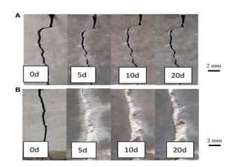
A self-healing concrete solution that utilizes the spore-forming ability of the alkaliphilic Bacillus Subtilis and thus act as a self-healing agent that will solve the problem of concrete structures deterioration well before the end of their service life as it will convert nutrients into limestone.
