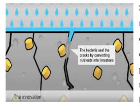
Self-healing concretes are being widely recognized as a remedial technique to improve the durability of concrete. Concrete strength has been enhanced by bio-technique based on calcite precipitation. Microbial cells achieved decent nourishment during the primary curing, as the binder mortar was porous. These microbial cells
